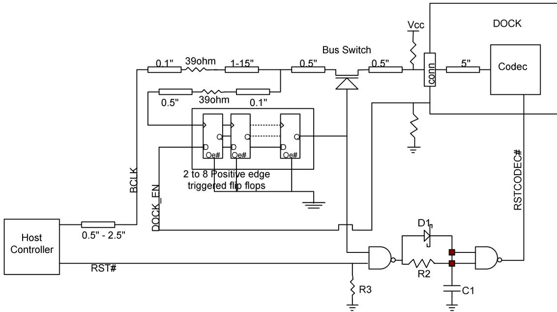
**Figure 15: Hot attach, synchronous solution**
