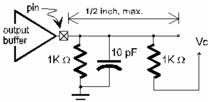
Figure 7: Slew rate and min valid delay
