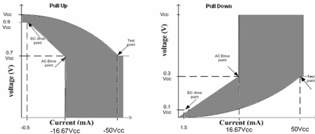
**Figure 4: V/I Curves for SDO buffers**
