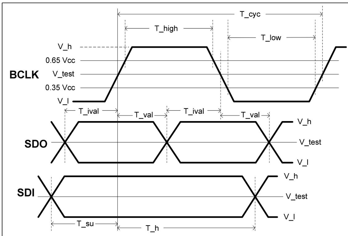
**Figure 9: Timing parameters as measured at the controller**
