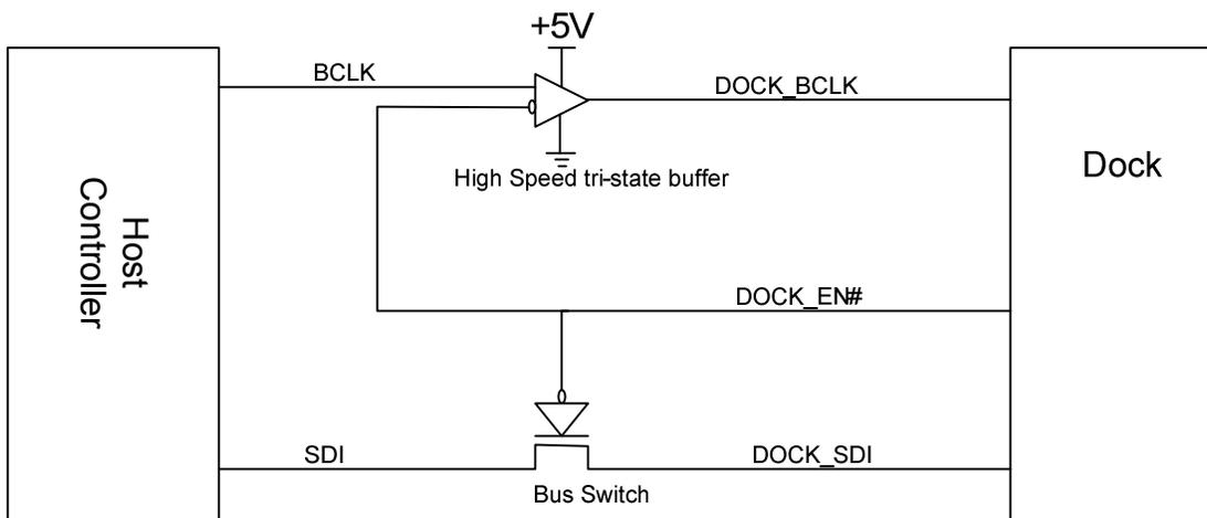
Figure 14: Hot attach Asynchronous solution
