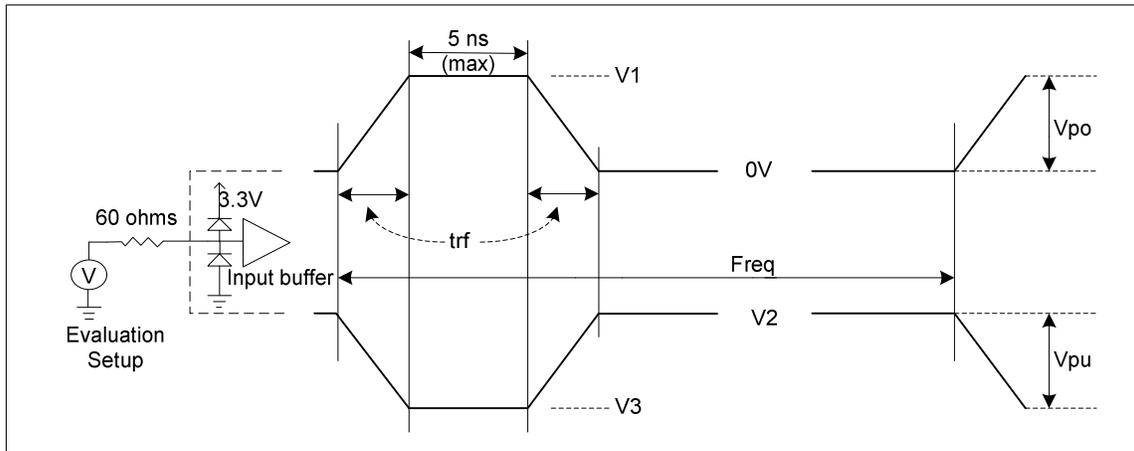
**Figure 3: Maximum AC waveforms for 3.3V signaling**
