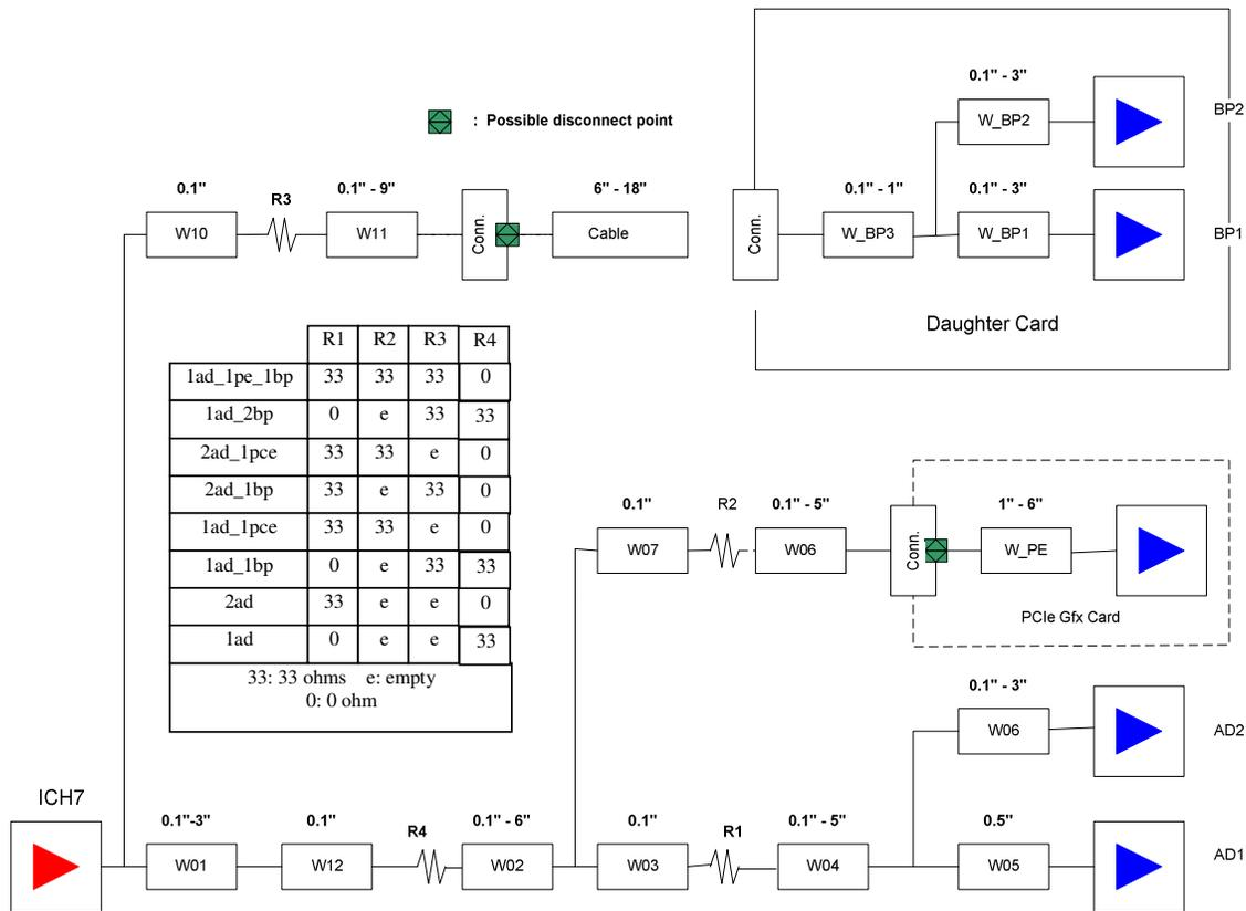
**Figure 11: Desktop platform configurations**
