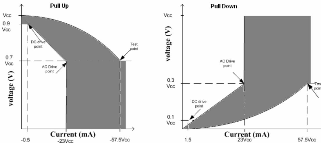
Figure 1: V/I Curves for SDO buffers
