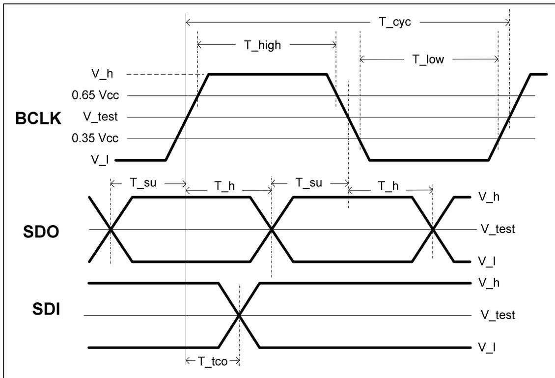
Figure 10: Timing parameters as measured at the codec
