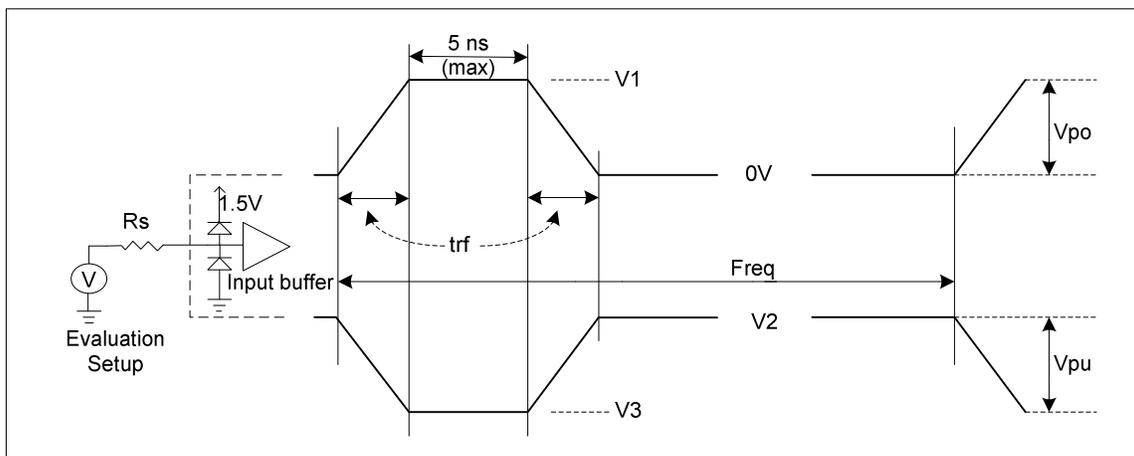
**Figure 6: Maximum AC waveforms for 1.5V signaling**
